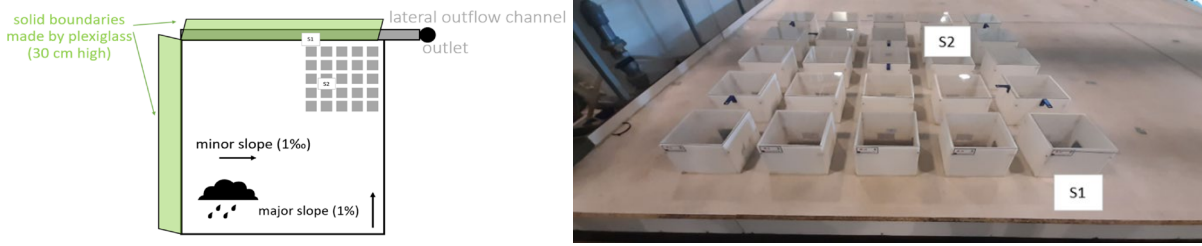
Figure 1: Laboratory setup of the scaled urban catchment model.
